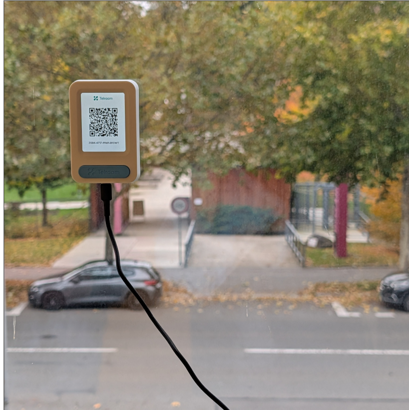
Figure 5: Telraam Sensor observing traffic at the front of the Palacký University Faculty of Science Building
